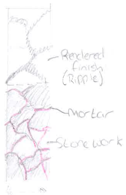
Cross Section of plastered Stone wall
